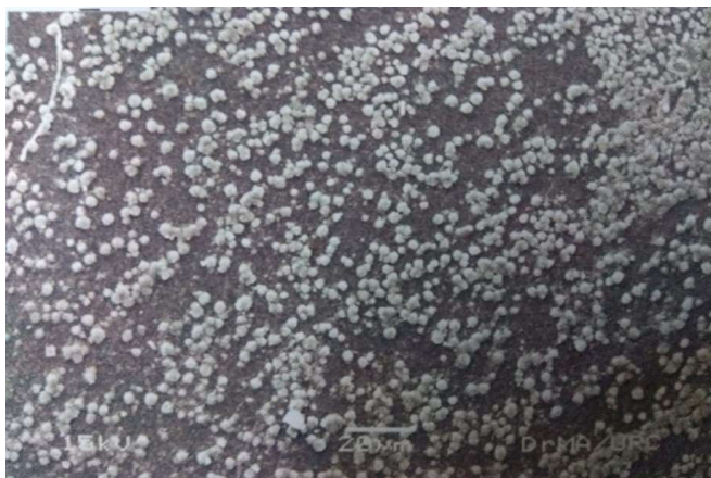
Figure 21: SEM micrograph of silver nanoparticles (Sample 4)
